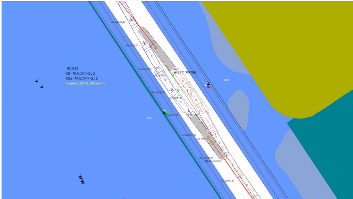
Figure 4. Two Design Containerships Meeting in the Proposed 700 ft Wide Houston Ship Channel
