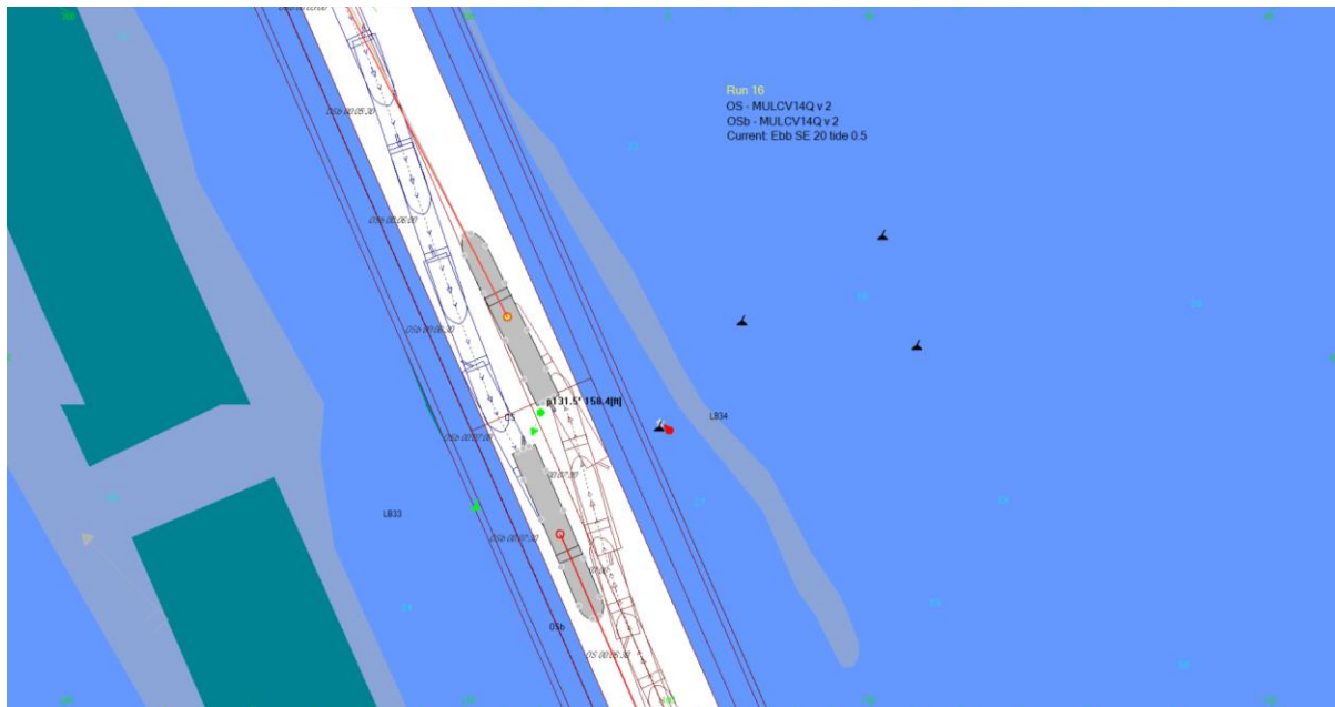
Figure 3. Two Design Containerships Meeting in the Proposed 650 ft Wide Houston Ship Channel
